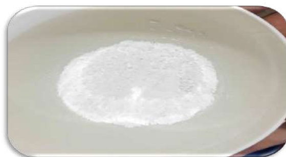
Figure.2: Synthesized MgO- nanoparticles(white powder).
